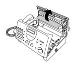
4 Close the print compartment cover (press down on both sides to make sure it clicks into place), and then close the operation panel.
